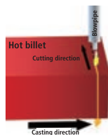
Illustration of billet cutting
