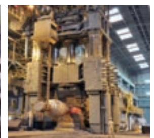
Forging machinery (forging press)
