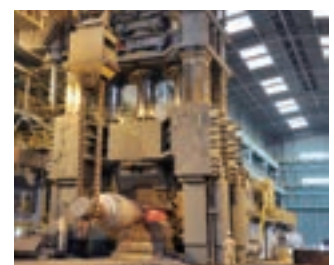
Forging machinery (Forging press)
