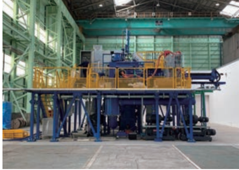
Vacuum melting furnace (VIM) (Precision castings production lines)
