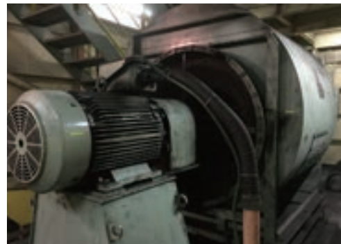
Motor cooling fan for finishing rolling machine
