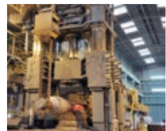
Forging Machinery (Forging press)
